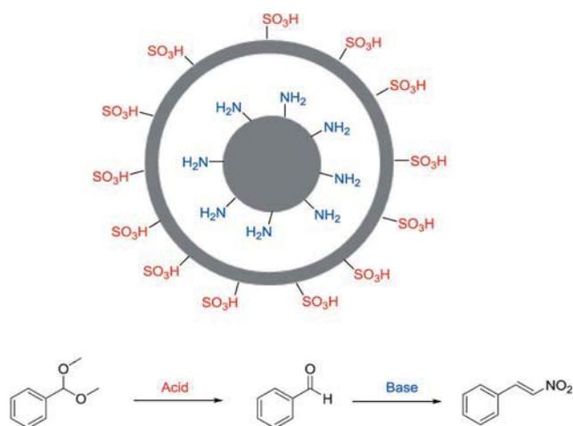
Figure 10. Deacetalization/Henry cascade reaction catalyzed by NH<sub>2</sub>@SO<sub>3</sub>H nanorattles.
