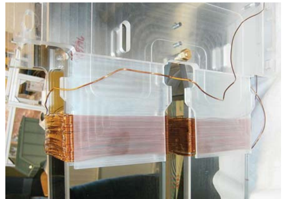
Fig. 8. Spin-flipper coils, wound around the two arms. The copper RF shieldings (removed for clarity) are located 3 mm around the spin-flippers.
