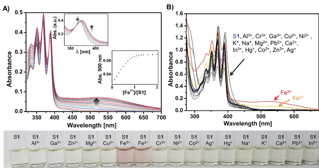
**Figure 1.** (A) UV–vis titration of **S1** ( $40 \mu M$ ) by  $Fe(NO_3)_3$  (0 to  $80 \mu M$ ) in DMF. The insets depict a zoom of the 370–420 nm window and the corresponding binding isotherm curve ( $\lambda = 530$  nm). (B) UV–vis spectrum and color of **S1** solutions ( $100 \mu M$  in DMF) upon the addition of 1.2 equiv ( $120 \mu M$ ) of different metal ions.
