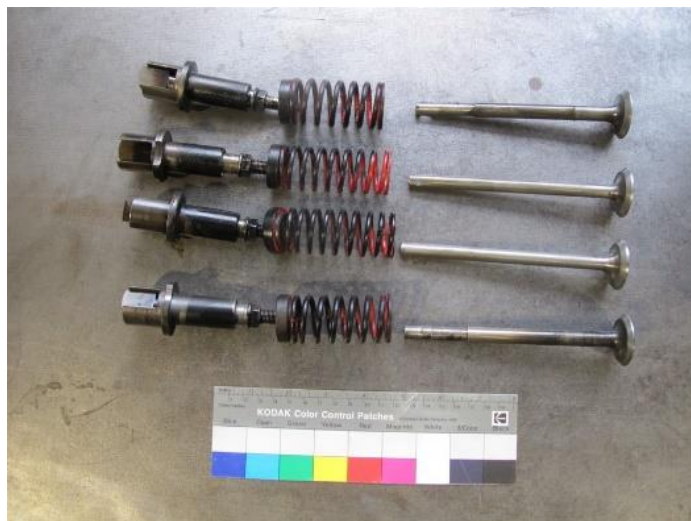
Figure 19 : Ensemble soupapes, ressorts, poussoirs et guides
