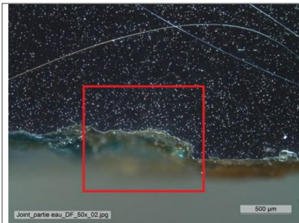
Fig. 10: Micrograph of the cross-section of the gasket, zone 2, shown on Fig. 5 unetched, dark field. SEM image Fig. 11 framed in red.
