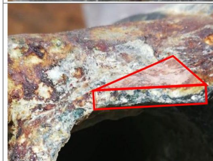
Fig. 4: Close up view of the Hispano water pump, with the exit pipe sampling area.
