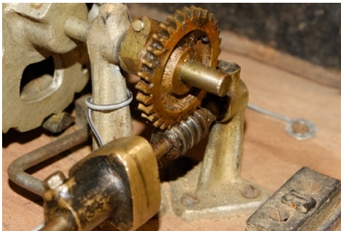
Fig. 115: Presence of old lubricant on the gears
