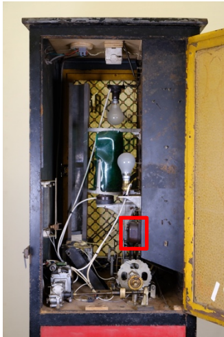
Fig. 77: Location of the buzzer inside the Green Ray, left view
