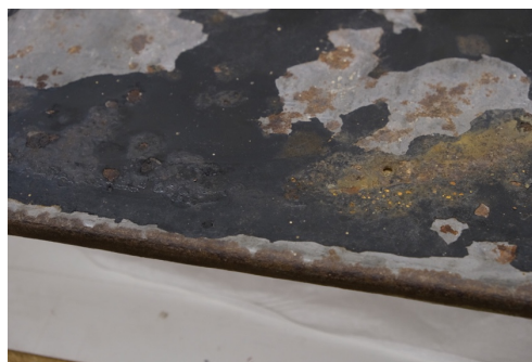
Fig. 142: The rust stains have been removed on the left with EDTA in gelled form
