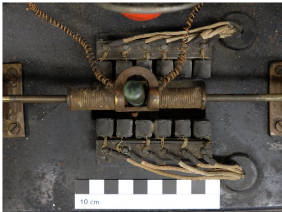
Fig. 89: View of the electro-magnet from above
