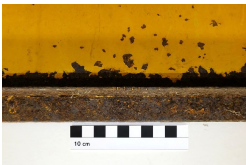
Fig. 102: Important loss of paint at the bottom of the lower right panel due to corrosion
