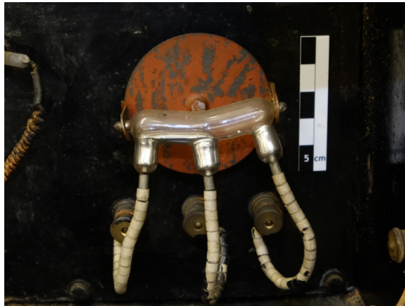
Fig. 39: Mercury switch on the front display
