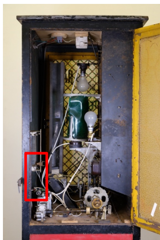
Fig. 72: Location of the rheostat inside the Green Ray, left view
