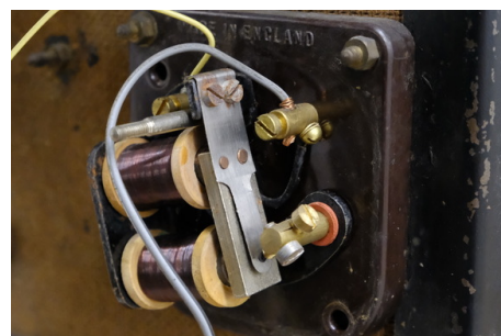
Fig. 134: Interior of the buzzer after treatment
