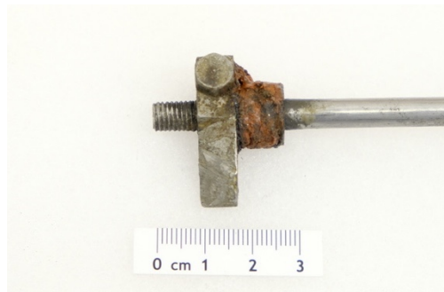
Fig. 118: Hook of the horizontal pen movement, with the oxidized rubber
