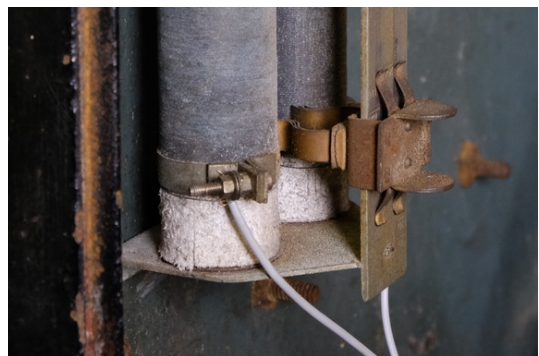
Fig. 123: Asbestos from the rheostat
