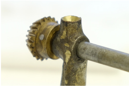
Fig. 119: Abrasion of the non-functional surface
