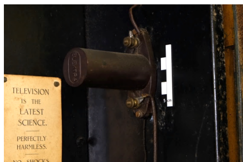
Fig. 114: Broken decorative component which was glued back, we see the adhesive has dripped
