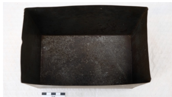
Fig. 138: Box after mechanical treatment and application of tannic acid
