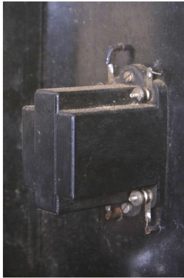
Fig. 87: d. Low Frequency (LF) Transformer
