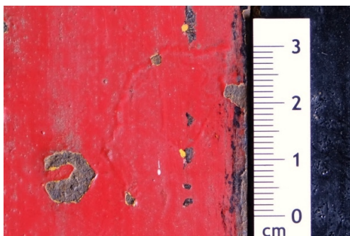
Fig. 96: We can notice a kind of filiform corrosion, black paint drips, and the yellow paint layer is visible
