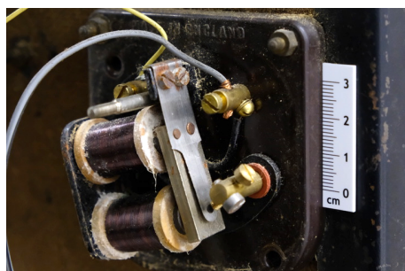
Fig. 133: Interior of the buzzer before treatment
