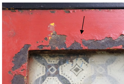
Fig. 140: Lifting of the paint layer on the upper right panel after treatment
