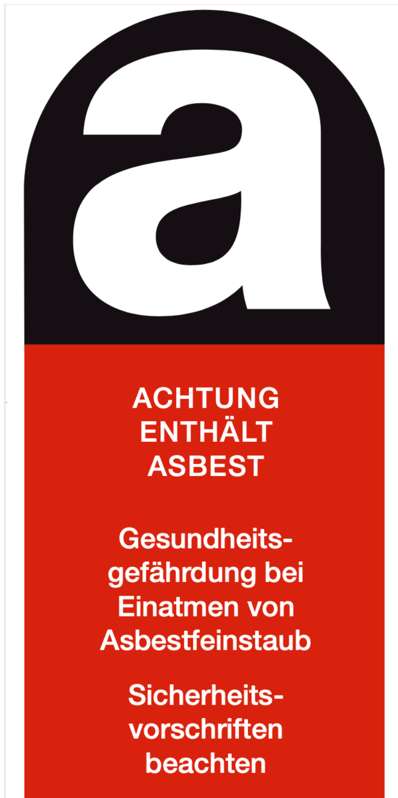
Fig. 180: Label which has to be put on the object in the presence of asbestos
