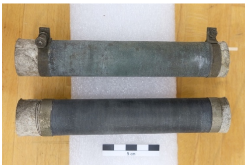
Fig. 129: Treatment of the wire coils, before (up) and after (down)
