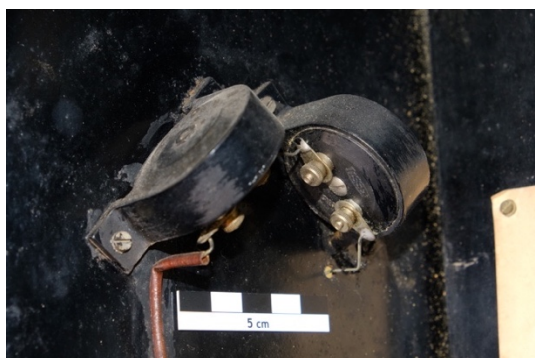
Fig. 84: a. Radio Frequency (RF) choke from the "Lissen" brand
