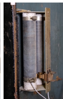
Fig. 74: Rheostat located on the back panel
