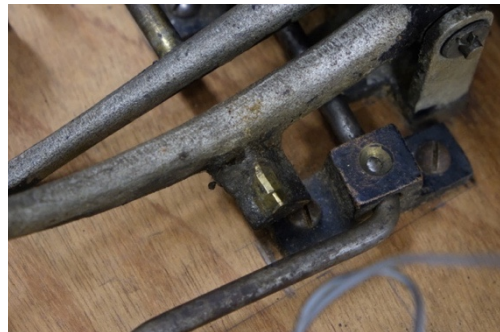
Fig. 116: The sensor of the mechanical switch is worn
