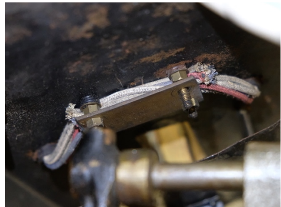
Fig. 90: Wiring of the electro-magnet on the inside, we can clearly see that it is cut
