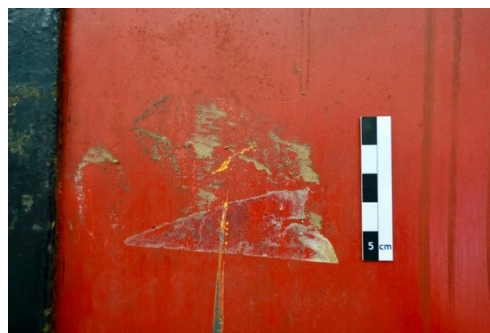
Fig. 97: Some of the residues from old labels or adhesive tape on the back panel
