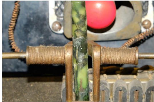
Fig. 120: Repair of the pen
