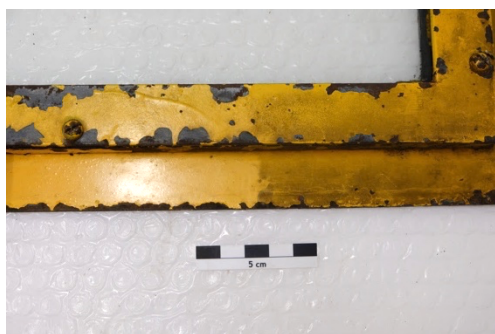
Fig. 145: After/before removal of the soiling on the inner side of the upper front panel
