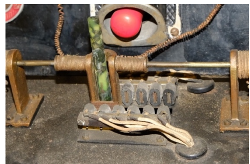
Fig. 31: Decorative cables and metallic elements simulating the presence of an electro-magnet
