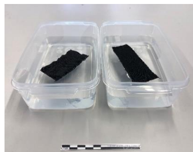
Figure 77 Soaking test of one big sample of warp (left) and one sample of weft (right) to evaluate the surface tension ©HE-Arc
