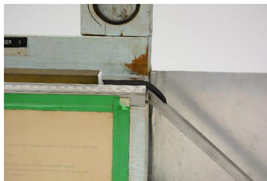
Figure 106 Modern sample touching the surface at 41.5 degrees, and ready to measure its bending length ©HE-Arc
