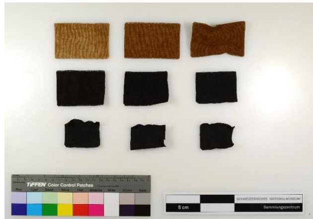
Figure 68 Modern samples. Carbonisation results varying the time (30min, 1h and 2h ; left to right), and temperature (300°C, 400°C and 500°C ; up to down) ©HE-Arc
