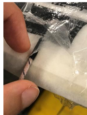
Figure 86 Attaching the thermocouple to a big warp sample pre-treated with 8% PEG 400 in deionised water ©HE-Arc
