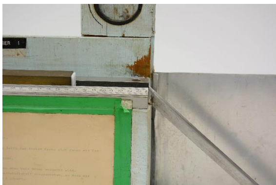
Figure 105 Modern sample on the starting point of the Shirley Stiffness tester ©HE-Arc
