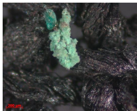
Figure 43 Detail of sample 3.01 under the microscope x5. Green deposit ©HE-Arc
