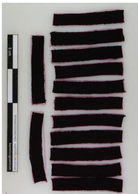
Figure 101 Modern samples from Group A: Visual comparison of the dimensions before (red line) and after freeze-drying ©HE-Arc
