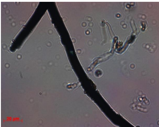
Figure 130 Single fibre from sample 2.19 under the polarised microscope x50, transmitted light ©HE-Arc
