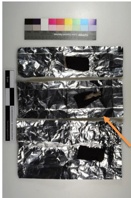
Figure 70 Results of the carbonisation varying the wrapping system. Two of the three samples burned (ashes visible with the naked eye) ©HE-Arc
