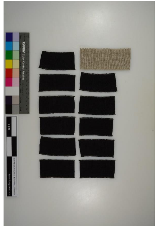
Figure 232 Carbonised big warp samples with an un-carbonised reference.
