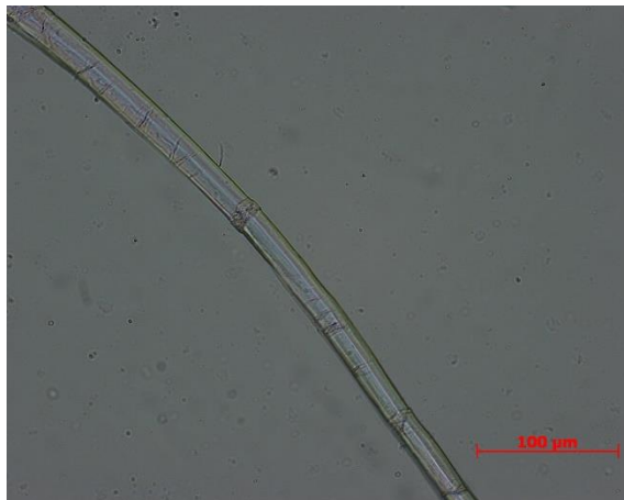
Figure 139 Modern flax fibre under polarised microscope x20, transmitted light ©HE-Arc
