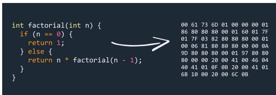
Figure 1 : Code en bytecode. <https://www.javascriptjanuary.com/blog/webassembly-neither-web-nor-assembly-but-revolutionary>
