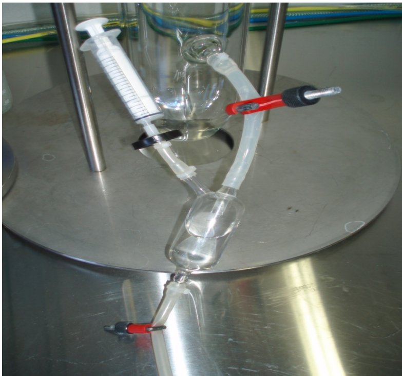
Figure 12 : sampler connecter au FBR sample port
