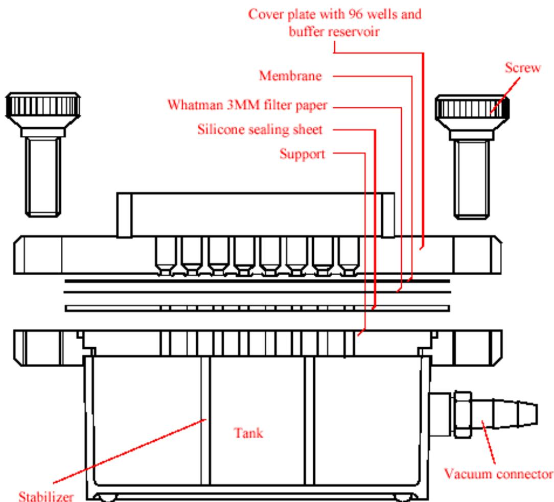
**Figure 21:** Set up of Dot Blot 96 (Biometra®) sandwich
