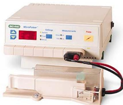
**Figure 20:** MicroPulser (Bio-Rad) used for electroporation of recombinant plasmid into *E.coli* supercompetent cells.
