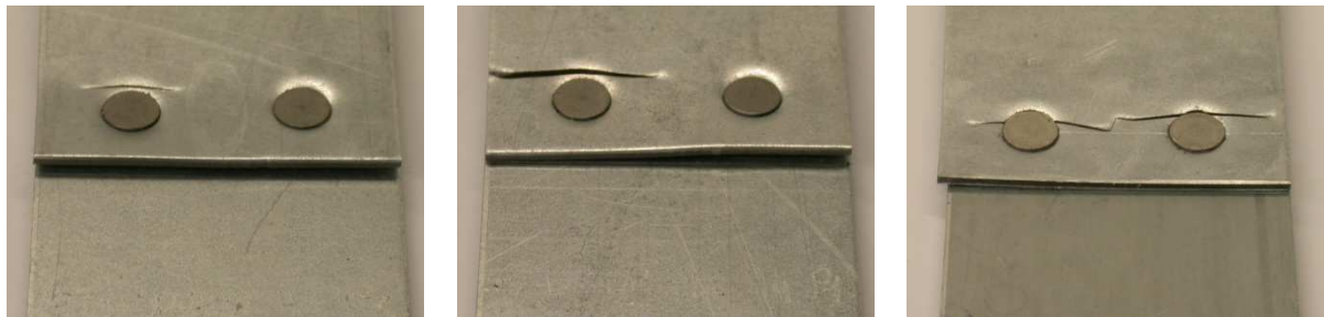
Fig. 93 Different HD2 fatigue samples: a) crack start b) crack grow c) two simultaneously cracks
