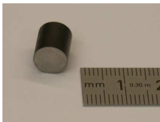
Fig. 15 Billet for a G rivet
