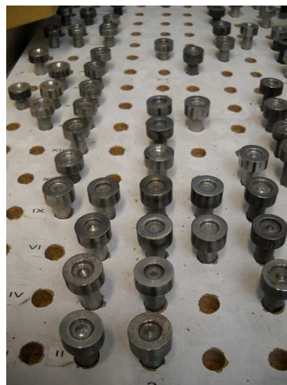
Fig. 19 Different dies for SPR developed at the FH Soest
