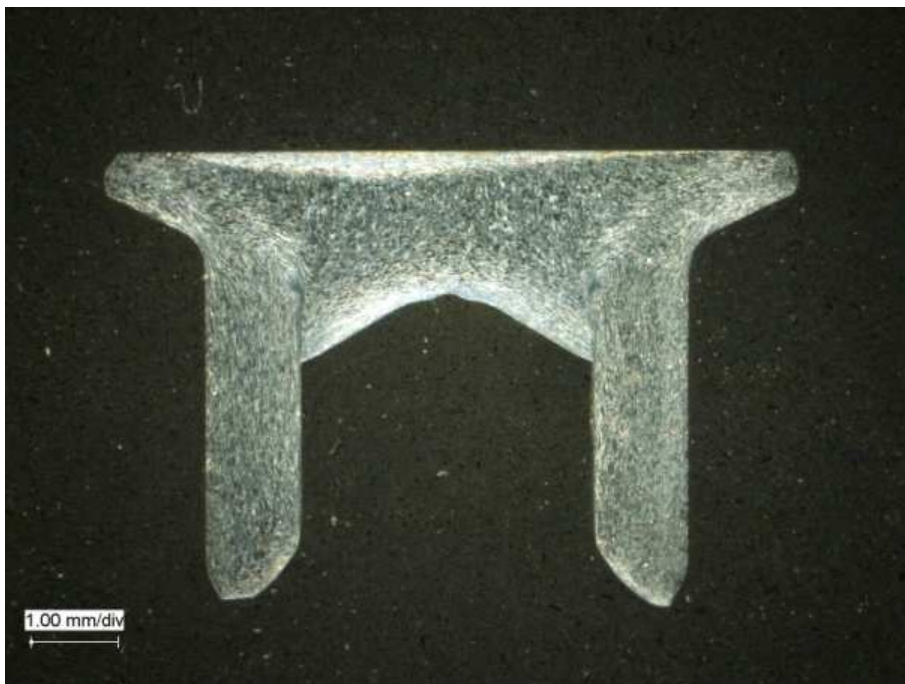
Fig. 55 Cold shaped G rivet
