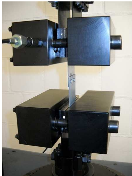
Fig. 51 Hydraulic clamping system of a resonant testing machine
