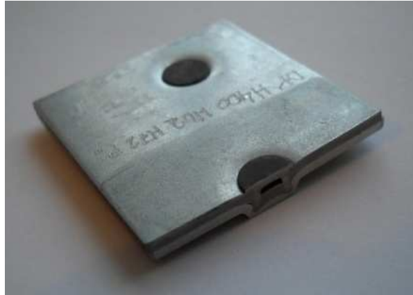
Fig. 39 Section of a HD2 rivet binding with DP-H400 combination
