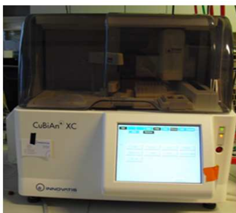
Figure 7: Picture of the CuBiAn XC analyzer. It is a compact version of a benchtop random access biochemistry analyzer (Innovatis, Bielefeld, Germany). It is applied for enzymatic and photometric assays.
