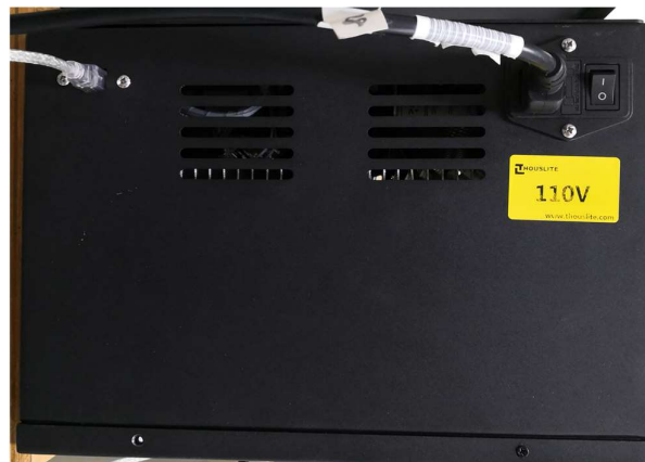
Figure 15: LED Cube interface, power supply and USB
