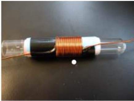
Figure 38 Photo of a coil made around a test tube [42]
