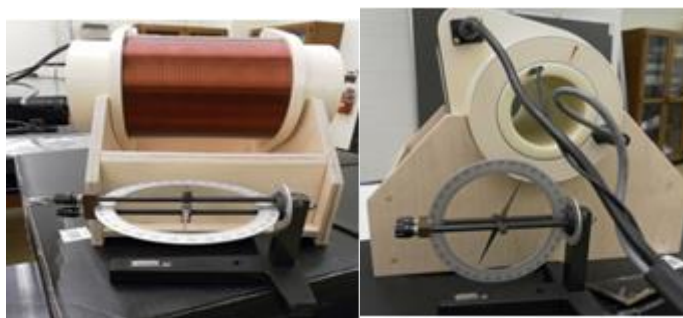
Figure 53 a) Alignment of the coil in quadrature of the earth's magnetic field. b) Alignment of the probe to the earth magnetic field B_0 [48]
