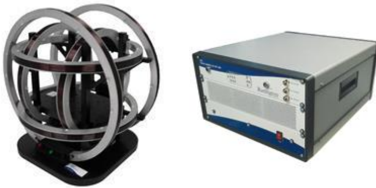
Figure 62 HC9 Helmholtz Coils and its PXI control system [56]
