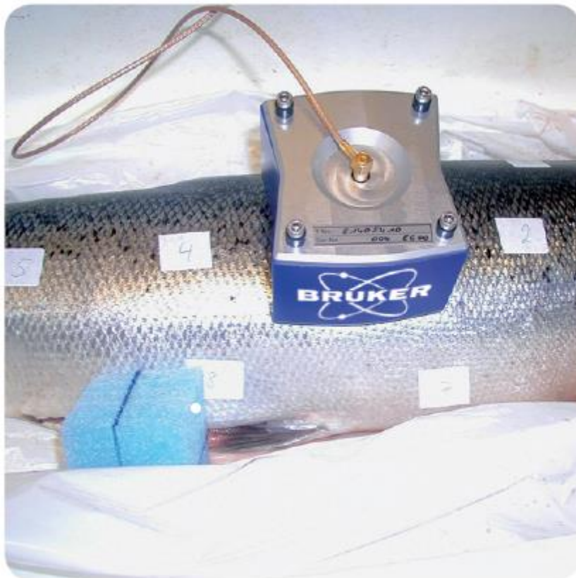
Figure 57 mq-ProFiler used in the determination of fat content in fresh fish and meat [52]
