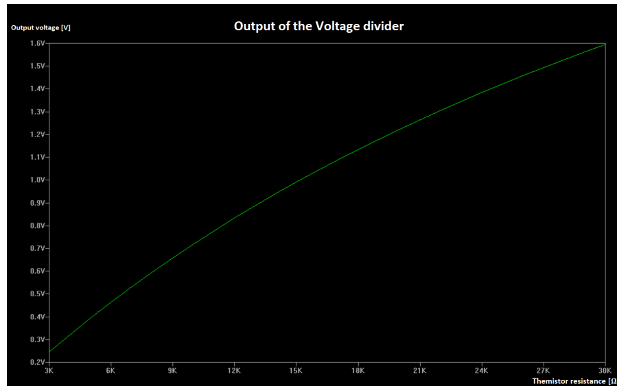
Figure 43: LTSpice simulation of the output of the voltage divider in function of the value of the thermistor resistance
