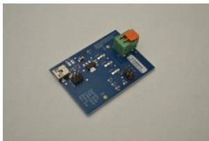
Figure 3: OpenROV Topside interface Board v2.6
