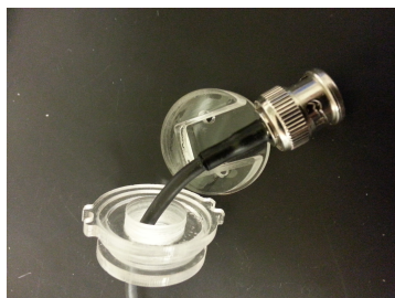
Figure 84: Endcap in two parts with cable
