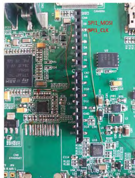
Figure 37 : Modification STM32F746G-Discovery
