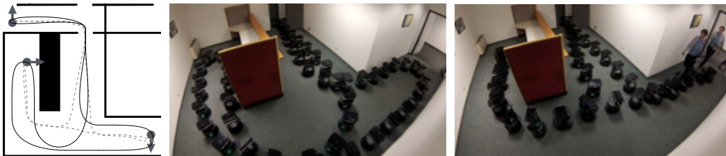
Figure 2.8. Left: qualitative comparison of the trajectories computed by our planner (solid black lines) and by the navfn planner (dashed grey lines). Center and right: the trajectories followed by the robot, which suffers slightly from inaccuracies in localization and in actuation (center: our planner, right: navfn planner).
