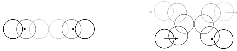
Figure 3.3. The worst case scenario considered to compute the upper bound M_s on the safety margin: two agents travel at maximal speed towards each other. Left : each needs at most v_{\text{opt}}(\Delta t + \tau) space to stop before colliding. Right : non-holonomic agents need additional space proportional to v_{\text{opt}}\tau_{\text{rot}} when they turn.
