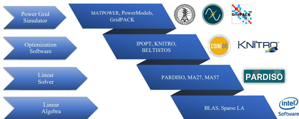
Figure 6.1. Software stack in power grid simulations.
