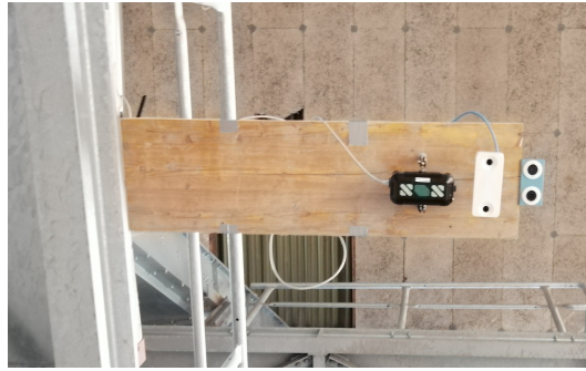
Figure 3.3 Sensors placement on the test rig : Hitachi, Vivotek (feeding Synology too) and Mobotix (from left to right)
