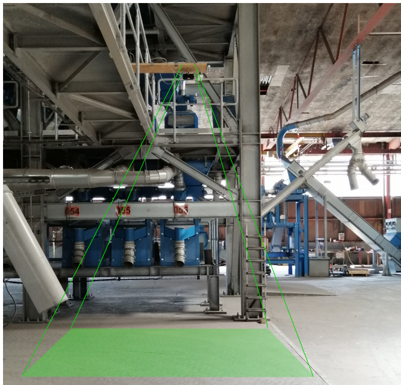
Figure 3.2 The Zone of Interest (in green) with the wooden board holding the sensors on top.
