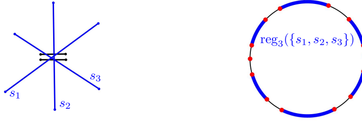
Figure 2.14. An instance of 5 segments (left), which has one region \text{reg}(\{s_1, s_2, s_3\}) , shown in blue, on the Gaussian map of the order-3 Voronoi diagram (right) with high complexity.
