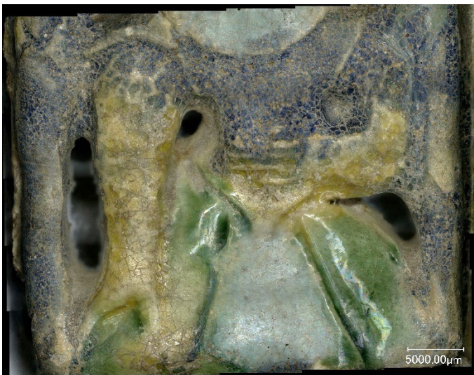
Figure 34: Degraded glaze on object 7216 © Scherrer, HKB
