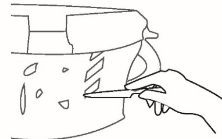
6. Cutting out the apertures
