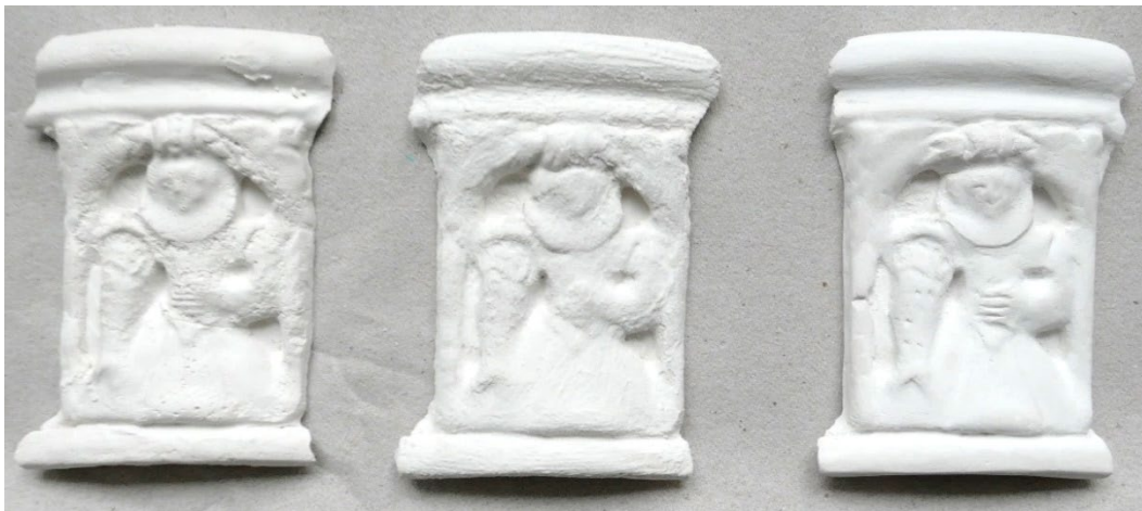
Figure 52: Plaster « copy » after casting (left), after applying Modostuc® (middle), and after sanding the Modostuc® (right)
