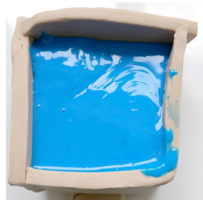
Figure 74: Liquid poly-additive silicone (WAGNERSIL 32N) is poured onto the object
