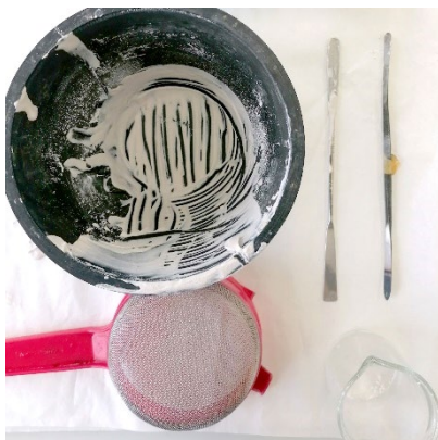
Figure 77: Materials for preparing plaster – rubber mixing bowl, sieve, flexible steel spatula, measuring cup
