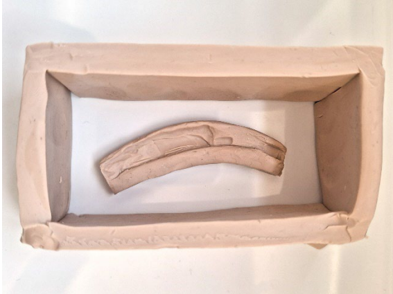
Figure 81: Plastiline® mold box, to mold the base piece
