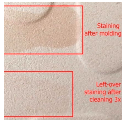
Figure 47: Comparison of the staining, before and after cleaning with White Spirit 100/140
