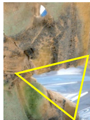
Figure 45: Example of an undercut between fragments
