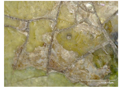
Figure 38: Crusts surrounding the crazing lines - 7216
