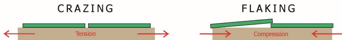
Figure 42: Glaze crazing and flaking processes
