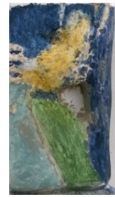
Figure 55: Replication of the colors, with Gamblin® on a surface finished with Paraloid®
