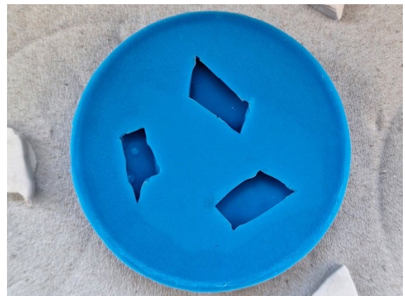
Figure 84: Silicone mold after trimming the excesses with small scissors
