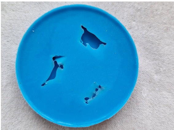
Figure 83: Silicone mold after curing and removing the Plastiline® pieces
