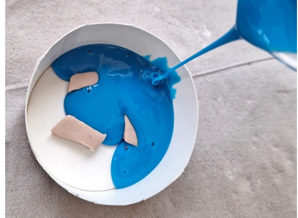
Figure 82: Pouring silicone (WAGNERSIL 32N) onto Plastiline® pieces, in the bottom of a cardboard cup
