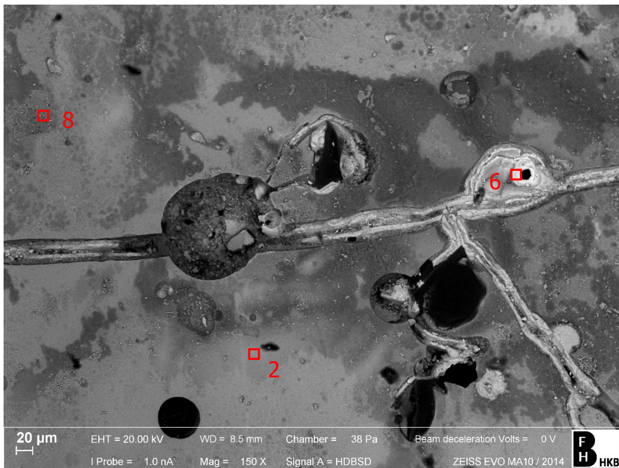
Figure 131: SEM picture of the light blue glaze, 150x magnification. Localization of the analysis points. © Nadim Scherrer, HKB
