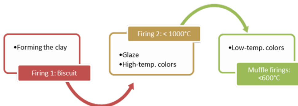
Figure 9: Firing process of glazed ceramics
