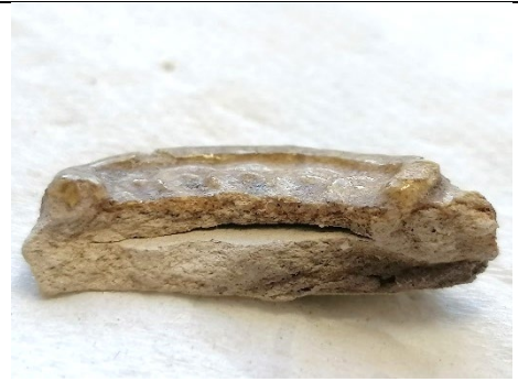
Figure 138: Separation between the applique and the underlying ceramic layer
