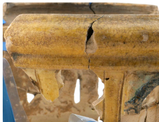
Figure 32: Glaze and surface lacuna because of breaking
