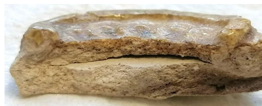
Figure 33: Separation between the imprinted motif and the underlying layer
