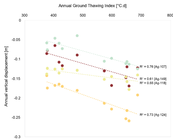
FIGURE 11 Contribution of GTI to annual vertical displacement for points Ag-107, Ag-118, Ag-124, and Ag-149 from 2006 to 2018. GTI is computed as the average of the seven location measurements in the glacier forefield [Colour figure can be viewed at wileyonlinelibrary.com ]
