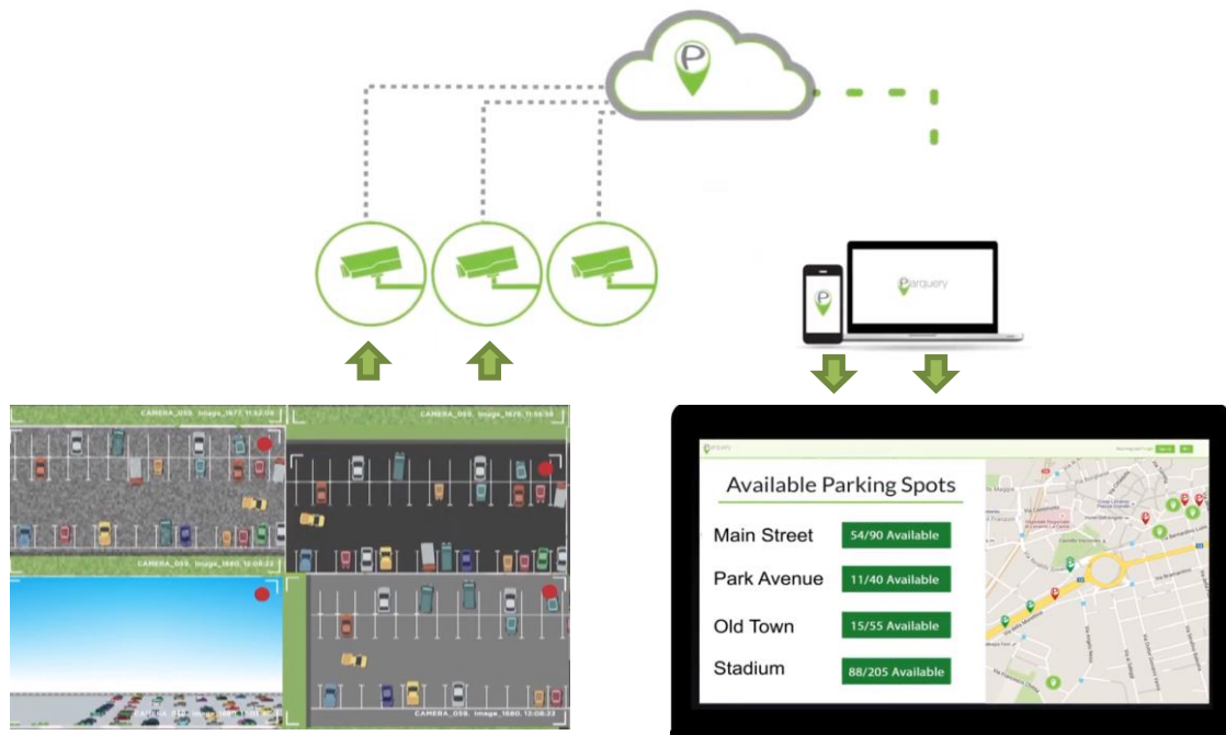
Figure 27, Parquery Parking System
